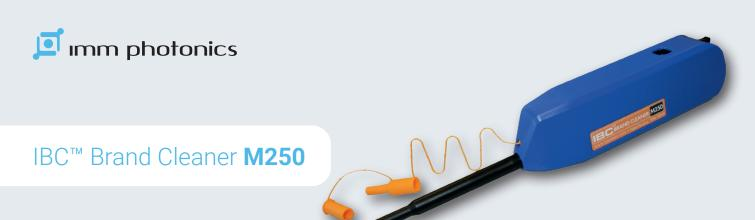
Patented fibre optic cleaner (US Conec) for cleaning 2.5 mm connectors such as SC, FC, ST for UPC and APC connectors. The cleaning pin turns while the cleaning band is drawn over the fibre end surface. This ensures that the fibre end surface is left clean after a single cleaning operation.
