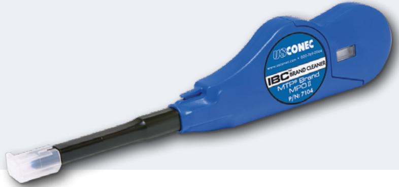
Patented fibre optic cleaner (US Conec) for cleaning MPO connectors. The cleaning pin turns while the cleaning band is drawn over the fibre end surface. This ensures that the fibre end surface is left clean after a single cleaning operation.
