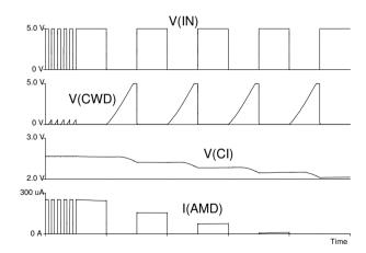
Figure 9: Watchdog, CWD open, f(IN) = 100 kHz  $\rightarrow$  10 kHz (1:1), CI = 470 nF, RSET = 10 k $\Omega$
