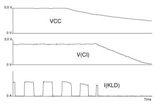
Figure 7: Turn-off behavior, f(IN) = 100 kHz (1:1), CI = 470 nF,  $RSET = 10 \text{ k}\Omega$
