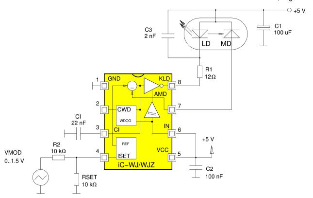
Figure 11: Analogue modulation during CW operation
