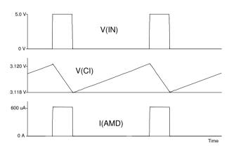
Figure 4: Steady-state averaging, f(IN) = 100 kHz(1:4), CI = 470 nF,  $RSET = 10 \text{ k}\Omega$
