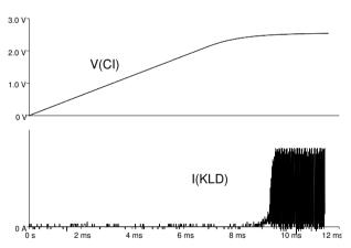
Figure 5: Turn-on behavior, f(IN) = 100 kHz (1:1), CI = 470 nF,  $RSET = 10 \text{ k}\Omega$
