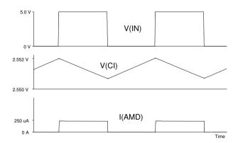
Figure 3: Steady-state averaging control, f(IN) = 100 kHz (1:1), CI = 470 nF,  $RSET = 10 \text{ k}\Omega$
