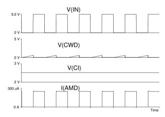
Figure 8: Watchdog, CWD open, f(IN) = 100 kHz(1:1), CI = 470 nF, RSET =  $10 \text{ k}\Omega$
