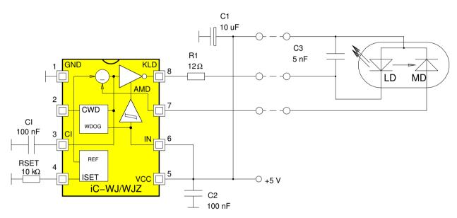
Figure 10: CW operation via cable
