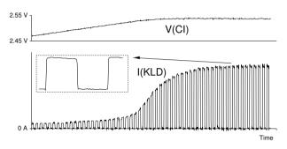
Figure 6: Turn-on behavior, detailed view f(IN) = 100 kHz (1:1), CI = 470 nF, RSET = 10 k $\Omega$
