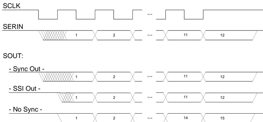
Figure 4: SOUT in the various modes of operation.
