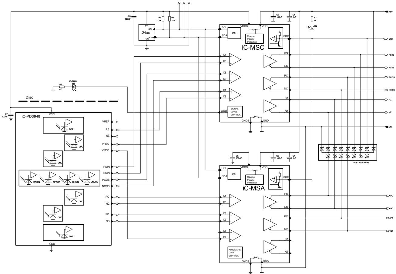
Figure 2: Application example motor feedback encoder utilizing iC-MSC and iC-MSA. Sine square plus cosine square LED power controlling with optional hysteresis by the advanced iC-MSC maintains the differential 1 Vpp signal of the S/C channel featuring 2048 CPR. The C/D channel with 1 CPR ensures its 1 Vpp differential signal by automatic gain control. In this setup, operation at high rpm speed and beyond iC-MSC's cut-off frequency is possible.
