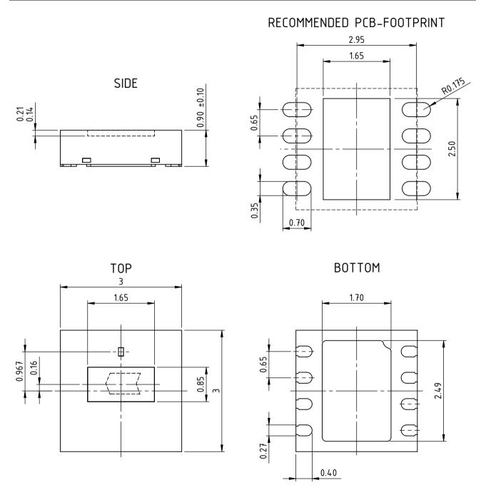
All dimensions given in mm. Tolerances of form and position according to JEDEC MO-229. Positional tolerance of sensor pattern: ±70µm / ±1° (with respect to center of backside pad). Maximum molding excess +20µm / -75µm versus surface of glass. drb\_pre1\_odfn8-3x3\_pxxxxx\_pack\_1, 15:1
