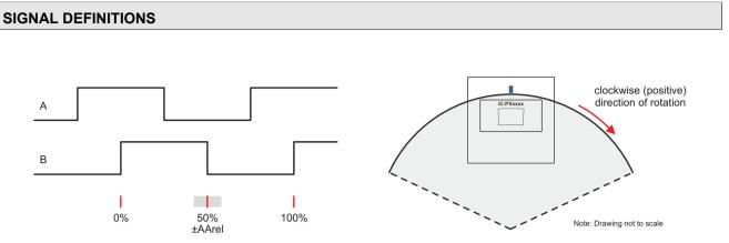
Figure 2: Signal definitions for clockwise (positive) direction of rotation.
