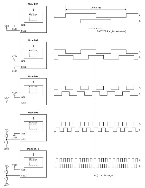
Figure 3: Illustration of operation modes selectable by pins SEL1 and SEL2.
