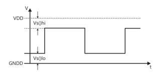
Figure 1: Digital Signal Levels.
