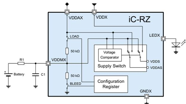
Figure 43: Circuit example for iC-RZ battery supply
