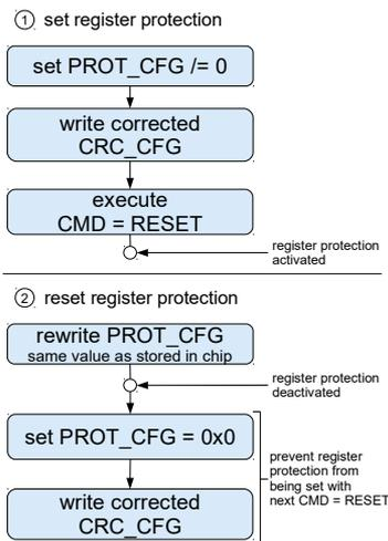
Figure 37: Enabling/disabling register protection
