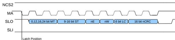
Figure 21: Extended SSI protocol
