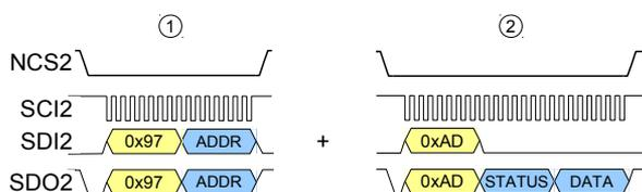
Figure 24: Read Register: set the read address (1) + command REGISTER status/data to read-out data (2)
