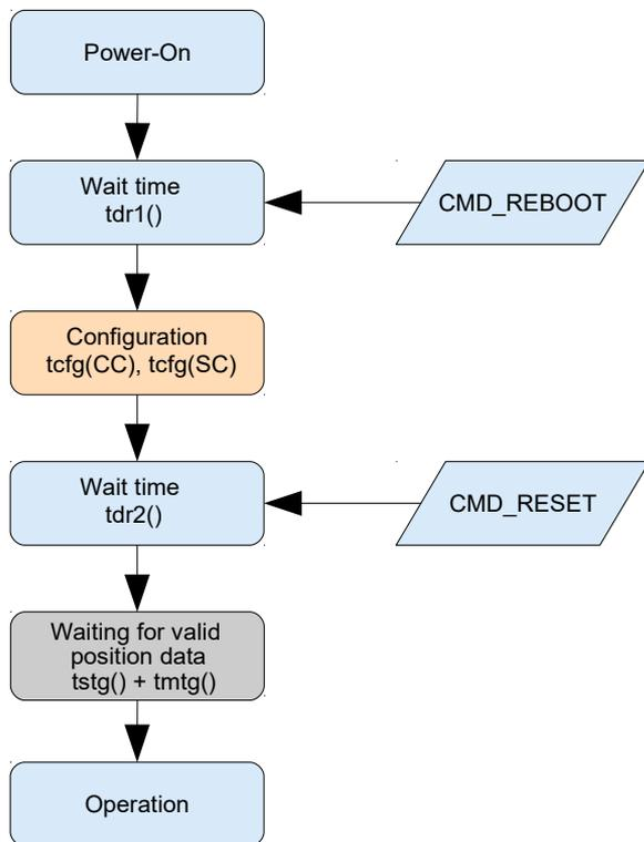
Figure 14: Overview of startup process
