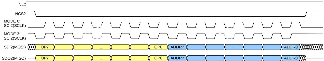
Figure 22: SPI protocol Safety Channel
