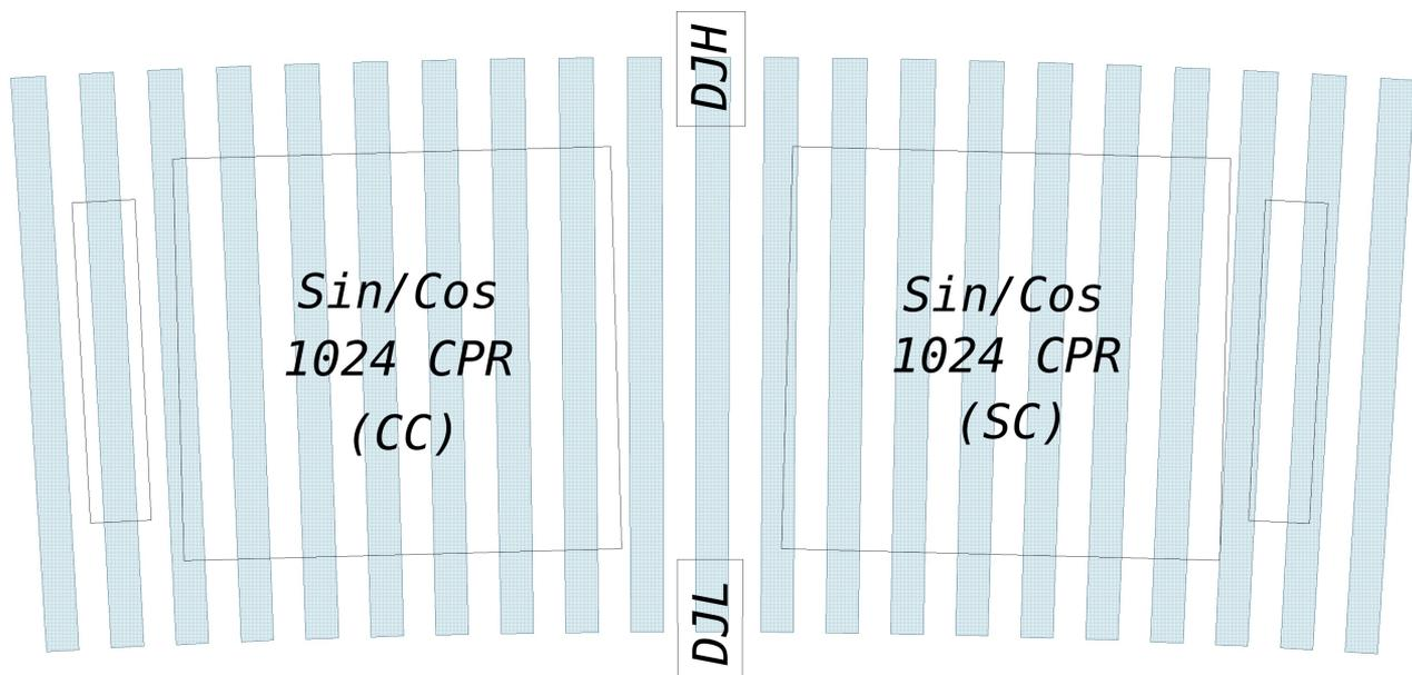
Figure 47: Alignment diodes DJH, DJL for radial alignment
