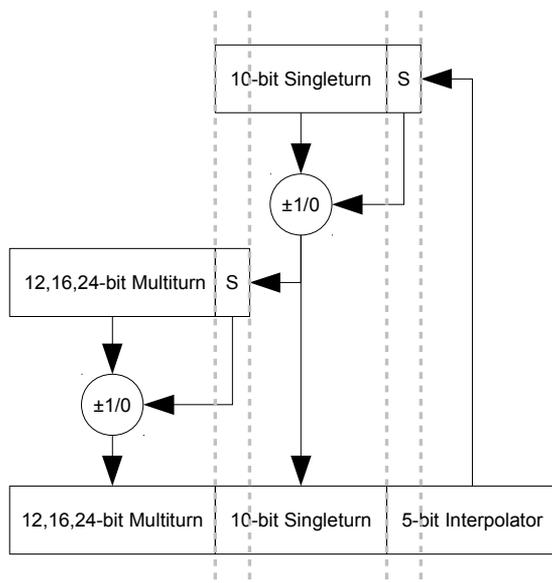
Figure 40: Synchronization position value
