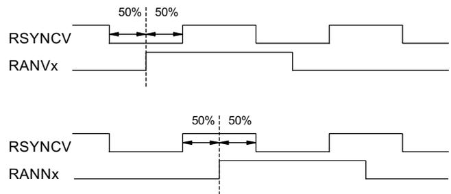
Figure 46: Signals for ideal tangential alignment
