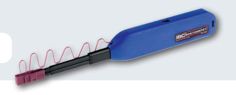
Patented fibre optic cleaner (US Conec) for cleaning MDC connectors. After each cleaning operation, the fibre cloth moves to make a clean section of cloth available for the next cleaning operation.
