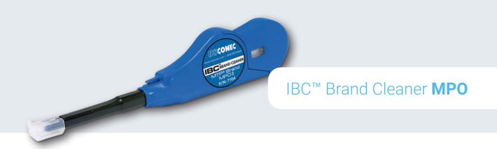
Patented fibre optic cleaner (US Conec) for cleaning MPO connectors. The cleaning pin turns while the cleaning band is drawn over the fibre end surface. This ensures that the fibre end surface is left clean after a single cleaning operation.
