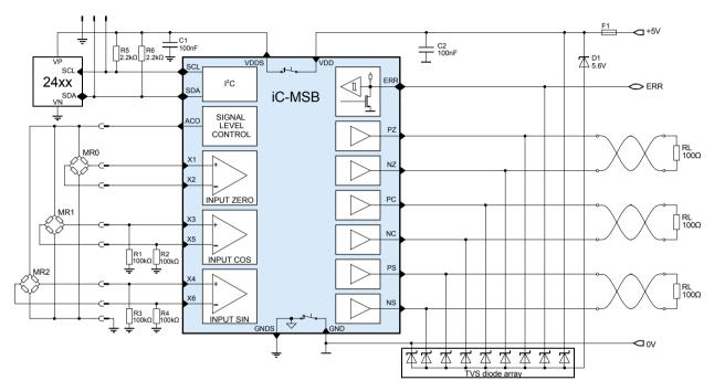
Figure 9: Example circuit for safety-related applications with iC-MSB<sup>SAFETY</sup>.
