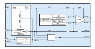
Figure 2: Signal conditioning input circuit.
