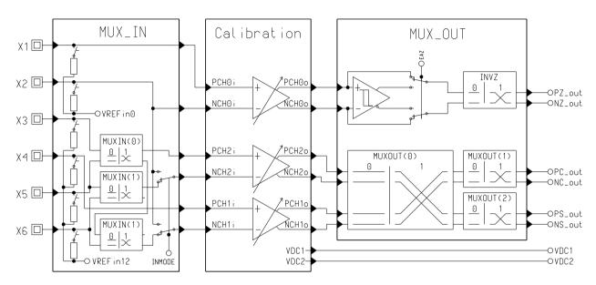
Figure 6: Multiplexer Schematics
