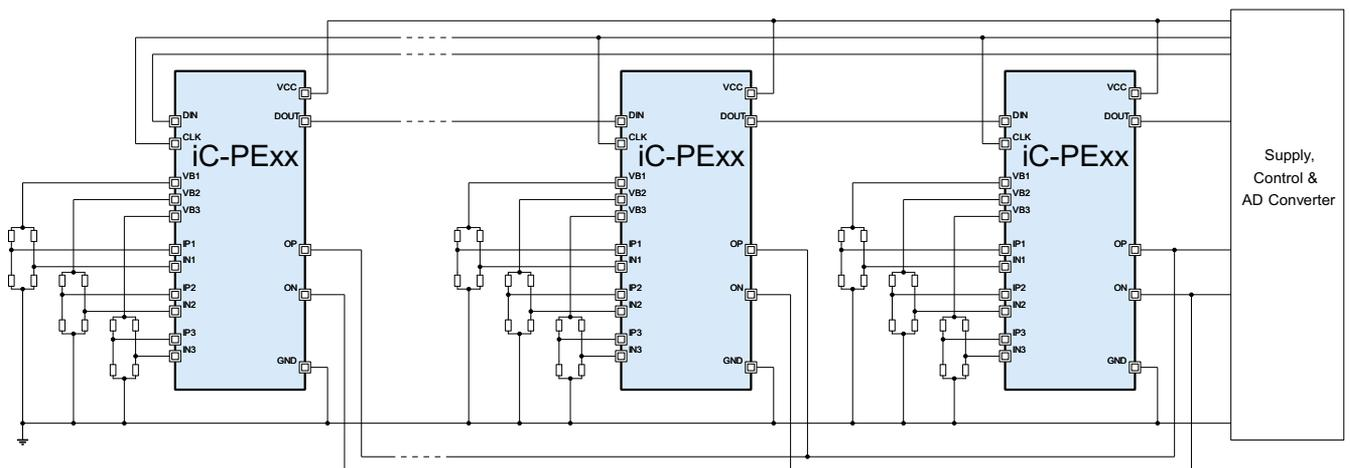
Figure 4: Chain configuration for sequential reading of multiple sensors
