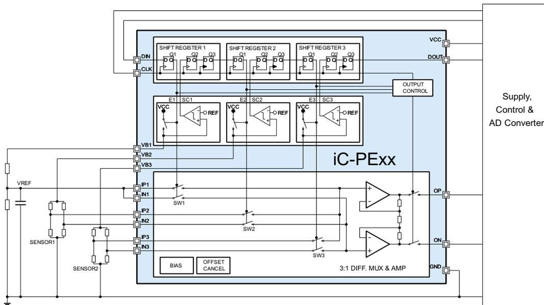
Figure 5: External offset compensation scheme
