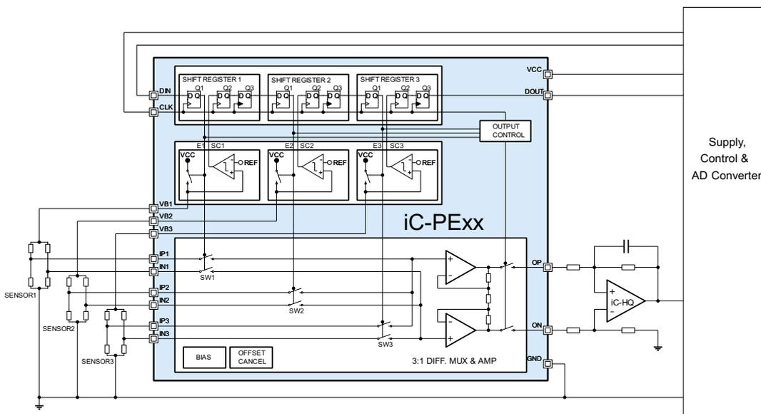
Figure 6: Instrumentation amplifier configuration with external op-amp
