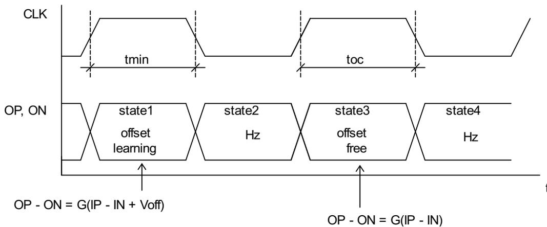
Figure 2: Internal offset canceling function timing characteristics
