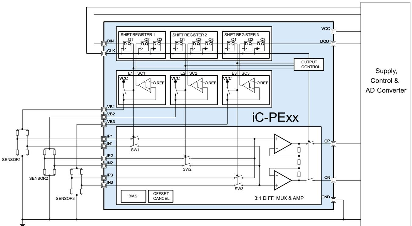
Figure 3: Single chip configuration for sequential reading of 3 bridge type sensors
