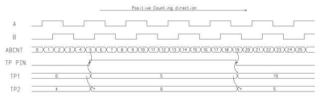
Figure 7: Function of TPI pin when TPCFG=11
