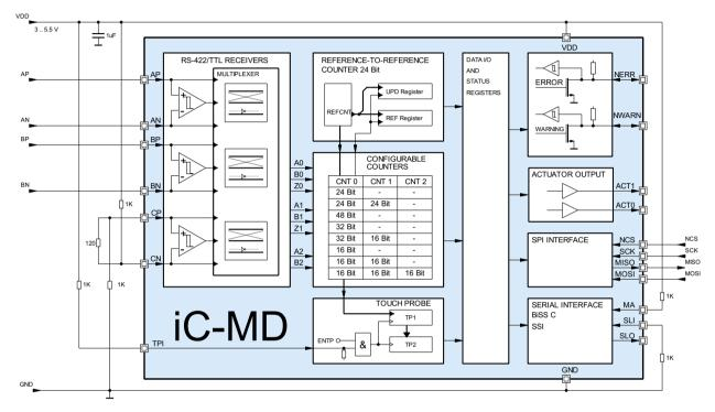
Figure 13: SPI only operation with unused constant pulled index input
