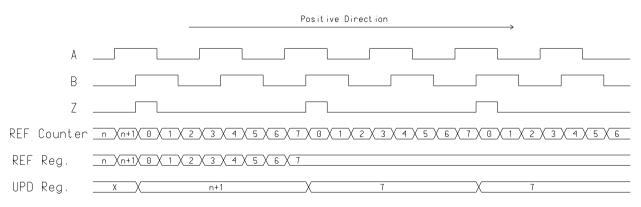
Figure 4: Zero-Codification: REF and UPD registers after activation of Zero Codification function
