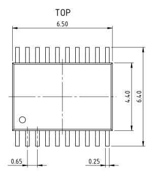
All dimensions given in mm. Tolerances of form and position according to JEDEC M0–153
