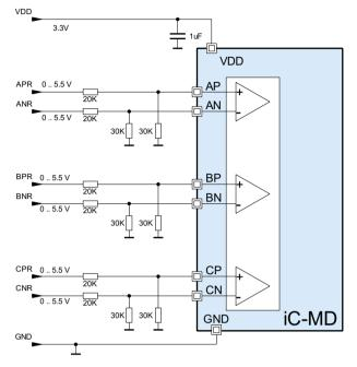
Figure 14: Input wiring for 5V signals with iC-MD supplied at 3.3 V.
