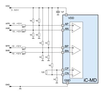
Figure 15: Input wiring for RS422 with +/- 12 V capability.
