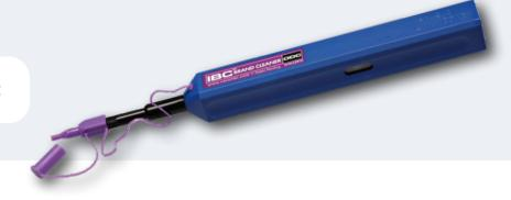
Patented fibre optic cleaner (US Conec) for cleaning 1.25 mm connectors such as ODC, URM for UPC and APC connectors. After each cleaning operation, the fibre cloth moves to make a clean section of cloth available for the next cleaning operation.
