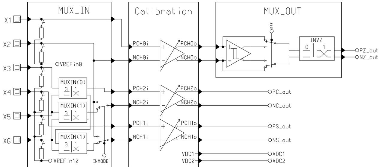
Figure 5: Multiplexer Schematics
