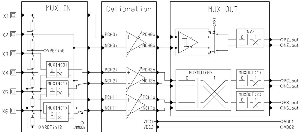
Figure 6: Multiplexer Schematics
