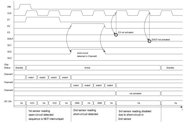
Figure 7: Example of open-circuit and short-circuit detection
