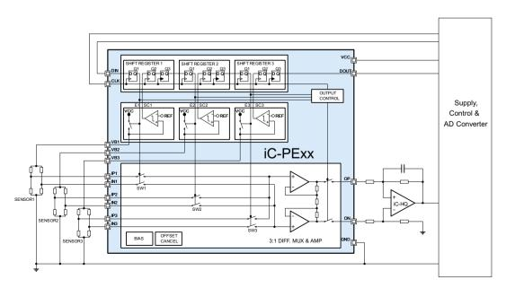
Figure 6: Instrumentation amplifier configuration with external op-amp
