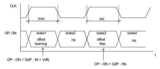
Figure 2: Internal offset canceling function timing characteristics
