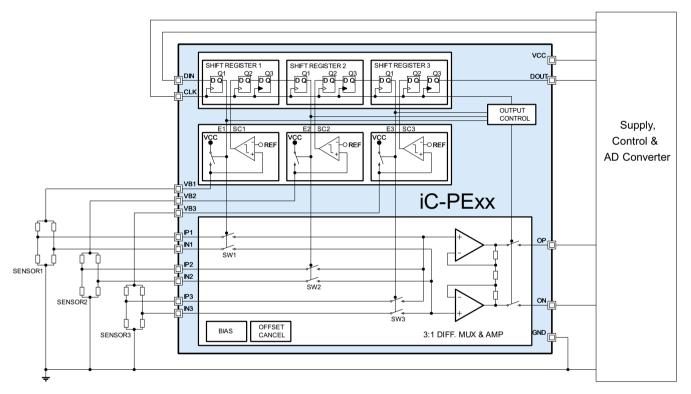
Figure 3: Single chip configuration for sequential reading of 3 bridge type sensors
