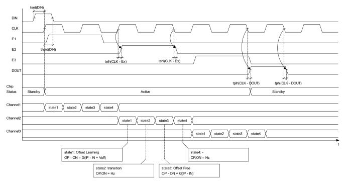
Figure 1: Timing characteristics
