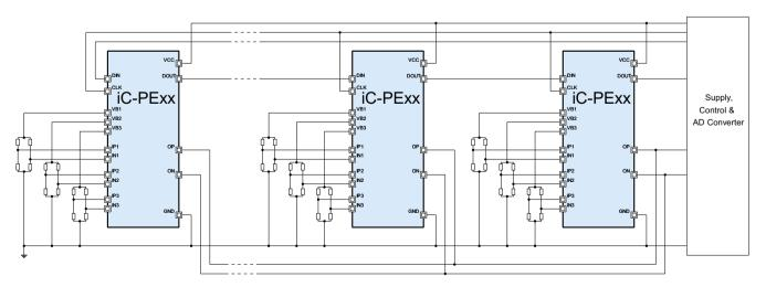
Figure 4: Chain configuration for sequential reading of multiple sensors
