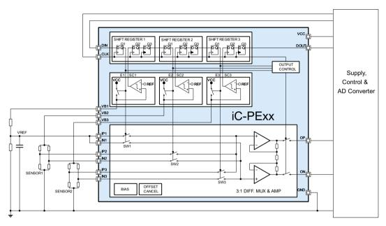
Figure 5: External offset compensation scheme
