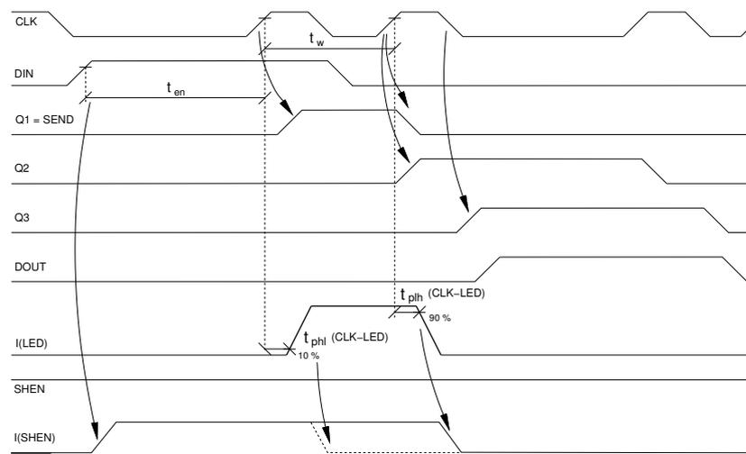
Figure 4: LED current pulse definition by clock signal (dashed line denotes  $I(\text{SHEN})$  in case of an interrupted LED path)
