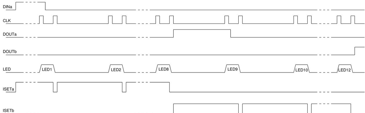
Figure 6: Signals of the chain configuration of Figure 5
