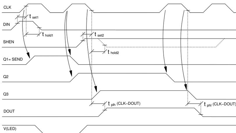
Figure 2: Timing characteristics
